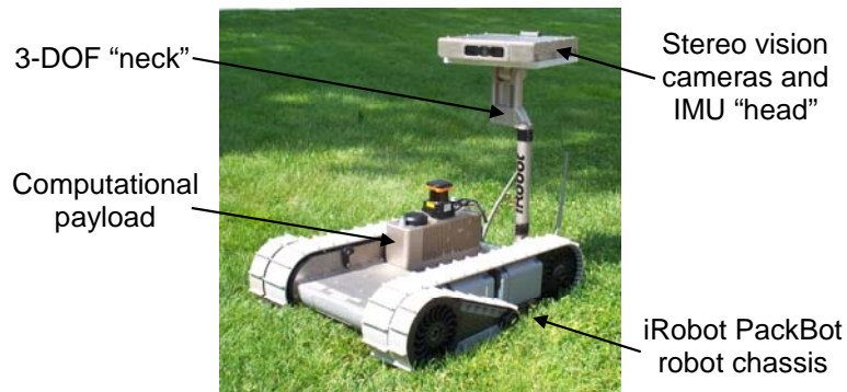
Fig 1 The robot is an iRobot PackBot chassis (tracked vehicle) augmented with stereo vision and additional computing power
