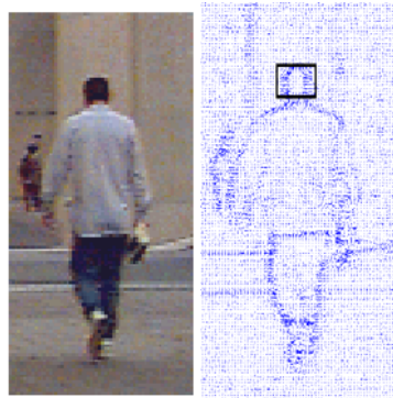
Fig 3 A typical pedestrian training image (left) and its gradient (right)
