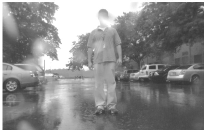
Fig 13 The detector continued to detect pedestrians even with rain drops partially obscuring the view
