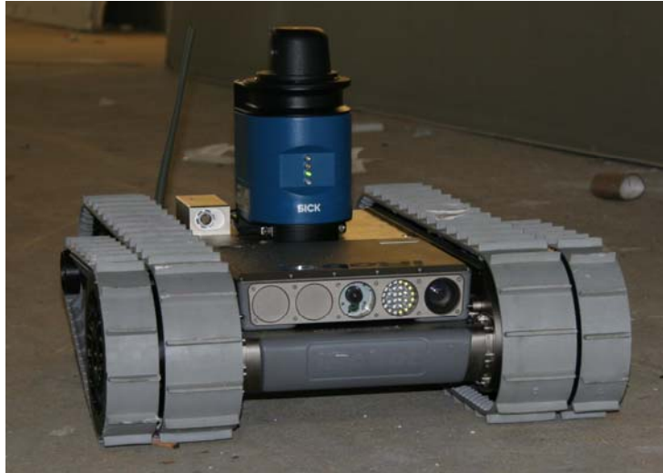
Figure 4 – The Mapping Kit is an iRobot PackBot augmented with a modular payload consisting of a LIDAR, a computational payload, and real-time mapping software.
