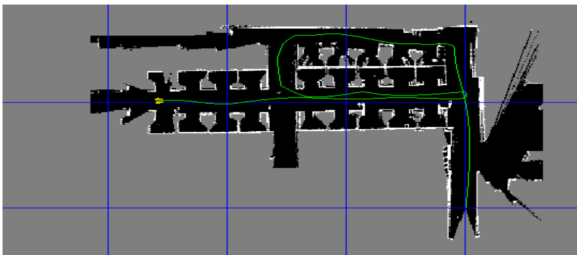
Figure 3 – The yellow robot was teleoperated along the green path to generate this map over a period of several minutes. The blue grid lines are spaced at 10m.
