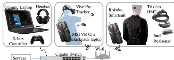
**Fig. 4:** Console (left), VR (middle), and AR (right) interfaces.
