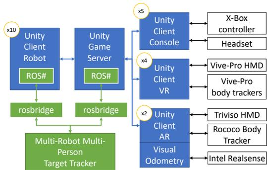
**Fig. 2:** The architecture includes ROS (green) and the Unity game engine [13] (blue). It consists of a Game Server and clients connected to the server. The clients include robot clients, and Console/AR/VR player clients.
