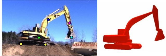
Fig. 1: The goal is to estimate the joint values and base pose of an articulated object, e.g. an excavator. In this case, links are tracked in an image stream (dots at left); recovering the joint values enables 3D reconstruction (right).
